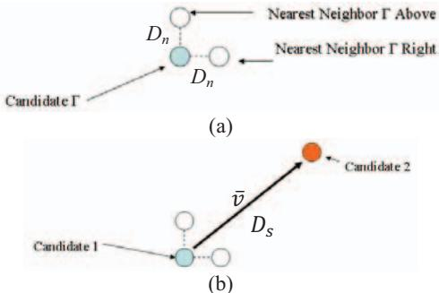
Fig. 4. (a) Estimation of gradient by  $\Gamma_L$  measurements of nearby points separated by neighboring-point distance  $D_n$ . (b) Jump to the next candidate point in the direction of steepest ascent by search distance  $D_s$  (reprinted from [5] for convenience).
