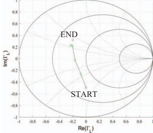
Fig. 6. Fast load-impedance optimization for output power from starting location  $\Gamma_L = 0.50/-90.0^\circ$ . A maximum  $G_T = 10.92$  dB was obtained at  $\Gamma_L = 0.38/122^\circ$  with 16 experimental queries.
