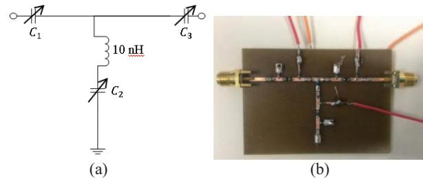
Fig. 1. (a) Design of 1.3 GHz tunable matching network, based on Fu [1], (b) implemented tunable-varactor matching network
