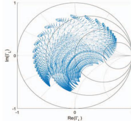
Fig. 2. Characterized load reflection coefficient states for the tunable varactor matching network
